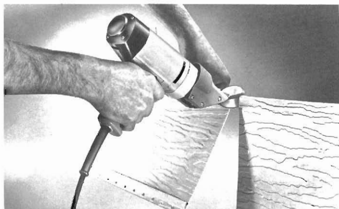
Large scissor blades cut lips and nailing strips with minimum distortion.
