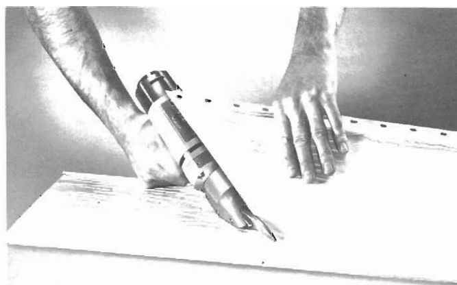
Makes precise angle cuts following a scribed line.
